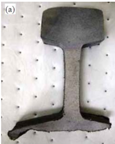
Figure 13: Corrosive Effects of Stray Current 9
