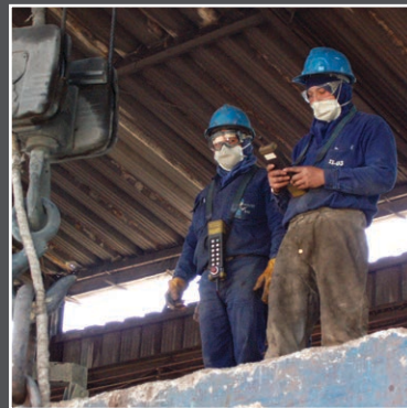
Radio Remote Control on an EOT Crane, El Salvador
