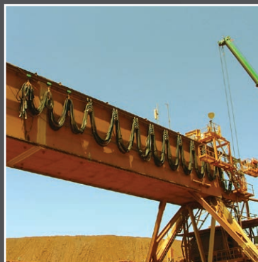
Festoon System on a Bridge Reclaimer, Australia
