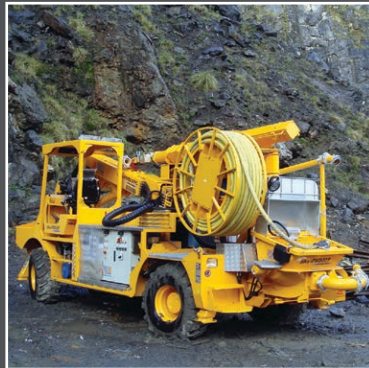
Motor Driven Hose Reel on a Shotcrete Machine, Spain
