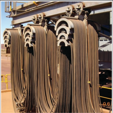
Festoon System on a Rail Car Dumper, Australia
