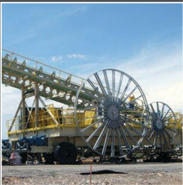
Motor Driven Cable Reels on a Radial Stackers, United Kingdom
