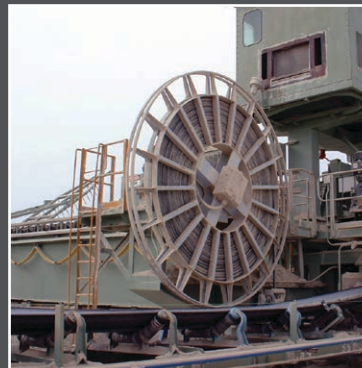
Level Wind Reel on a Stacker/Reclaimer, USA
