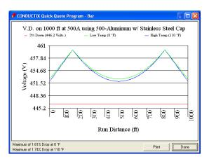
Figure 4: Two power feeds optimally located. The voltage drop remains under 3%, without the need to increase conductor capacity. A load positioned between the two feed points is supplied by both power feeds.
