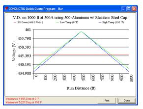
*Figure 2:* - Same parameters as Fig. 1, except with a 1000 foot (304.8 meters) system. Note that the voltage drop is now greater than the recommended 3%.
