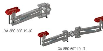
For systems up to 600 volts with straight runs and curves to 18" minimum radius. Assemblies have 19" pigtails (not shown in the illustration). Choose standard bottom entry or lateral-mount versions.
