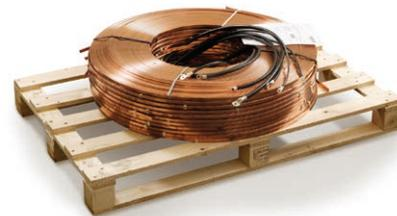
Conductor strip package ready for assembly
