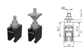
Suspension is carried out using freely swivelling clip-on Hanger Clamps that are self-aligning and permit low-friction slipping in case of thermal expansion. Hanger Clamps are available with hex nuts or square nuts for the mounting of Support Arms / C-rails (see installation accessories).
