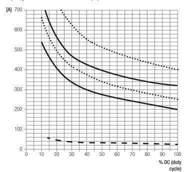
The load current of the conductor rail can be increased for shorter duty cycles. **Note:** When comparing the rated currents of rails from different manufacturers, always take into consideration the reference ambient temperature and the duty cycle! Consumptions with 100% duty cycle such as lighting, air conditioning or magnetic grippers must be taken into consideration. 100% DC  $\triangleq$  t  $\geq$ 10 min. (according to EN standards)
