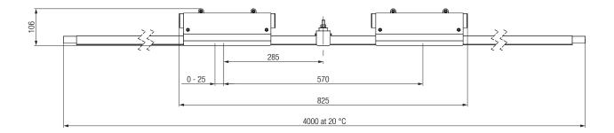
To compensate for changes in length due to temperature for systems > 100 m or segments connected between two fixed points such as Pickup Guides on both ends of the segment, or in curves (natural fixed points), expansion elements are needed to absorb the change in length. The expansion element has two expansion points, each of which can absorb 25 mm of expansion. The expansion elements / expansion unit parts are, like the rails, designed as 4 m standard components.
