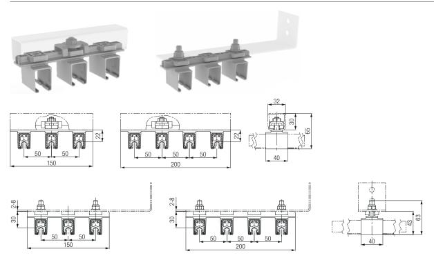
Compact Hanger Clamps for fast assembly of 3 or 4 rails indoors. Available for surface mounting or insertion into Conductix-Wampfler C-rails and mounting brackets in galvanized or stainless steel with 30 mm rated dimensions.
