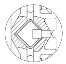
In installations with intersections, it is impossible to move the standard PE conductor Current Collector (with deflector angle) through the Pickup Guide. Thus the PE conductor Current Collector is used for intersections whose holders are equipped with a bolt for the Towing Arm. This fixes the position of the PE conductor Current Collector by being inserted into a hole drilled into the Towing Arm using the Drilling Jig listed below.
