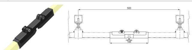
Air Gaps are used for the galvanic isolation of sections, such as maintenance segments that can be supplied with power and turned off separately. For each separation point, two Air Gaps must be mounted at a suitable distance to avoid power carryover through the Current Collectors.
