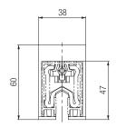
End Caps are used as a rail terminator and contact protection and are fastened to the rails using clamping screws.
