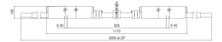
To compensate for changes in length due to temperature for systems > 200 m or segments connected between two fixed points such as Pickup Guides on both ends of the segment, or in curves (natural fixed points), expansion elements are needed to absorb the change in length. The expansion element has two expansion points, each of which can absorb 25 mm of expansion. The expansion elements / expansion unit parts are, like the rails, designed as 5 m standard components.
