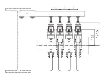
For installations without transfer points the current collectors for vertical and horizontal operation can be staggered. This way the center distance between two conductor rails is reduced by 10 mm.
