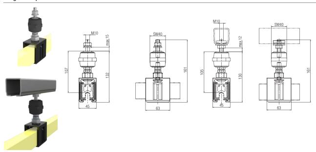
Suspension is carried out using freely swivelling clip-on Hanger Clamps that are self-aligning and permit low-friction slipping in case of thermal expansion.
