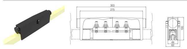
Rails are connected using compact screw connections. The rail connections must have exposed metal on all contact surfaces and be coated with a thin layer of contact grease (Part no. 080021) to protect against corrosion. When mounting clamping screws, use a torque wrench to achieve correct tightening torques.
