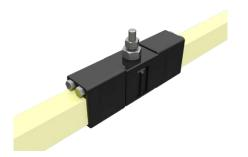
The rails are fixed in one place with Anchor Clamps and can expand freely from that point out. The fixed point is mainly for single feed applications attached close to the power feed or in the center of the conductor rail system. If multiple fixed points are planned, for example at intersections or curves (natural fixed point), the segment between the fixed points must be decoupled using Expansion Units. Clamps are fastened with a clamping cone on the rail insulator.
