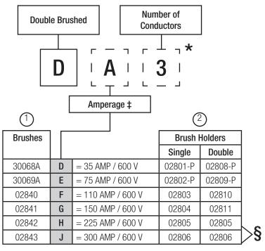
**‡** Multiple Amperage Sections are possible.
