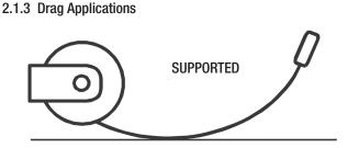
2.1.3.1 The reel is mounted on a stationary object and is required to drag the cable over the surface to the reel. A ratchet and/or ball stop may be desired.
