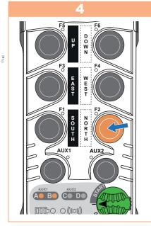
Press **F2** button on the transmitter to stop the scan. LED A indicates the tenths and B the units of the best radio channel found.
