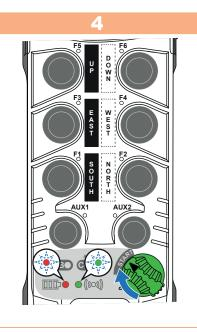
Confirm the value by turning the ON/OFF switch to START. During transmission: • Battery and radio LEDs flash alternately
