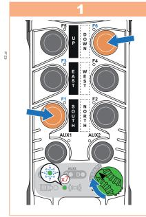
Turn **ON/OFF** switch to the I (ON) position. Ensure the LEDs A through D turn on and then off. Then press and hold the **F1 and F6** buttons and turn the **ON/OFF** switch to **START**:
