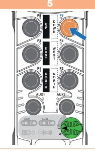
To disable the mode, press the **F6** button. This returns to the fixed radio channel setting (refer to Chapter **8.7.1**).
