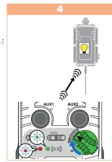
Confirm the selected status by turning the **ON/OFF** switch to **START**. During transmission: • Battery and radio LEDs flash alternately • Receiver light turns on.
