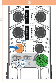
The passive stop delay is factorysetted to 0.5 sec and the LED B flashes 1 time.
