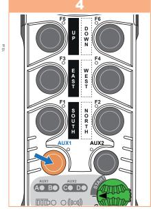
Press the **AUX1** button to scroll the power from 1 to 4.
