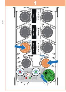
Turn **ON/OFF** switch to the **I** (ON) position. Ensure the LEDs A through D turn on and then off. Then press and hold the **AUX2 and F1** buttons and turn the **ON/OFF** switch to **START**: Battery and radio LEDs flash once in a loop.
