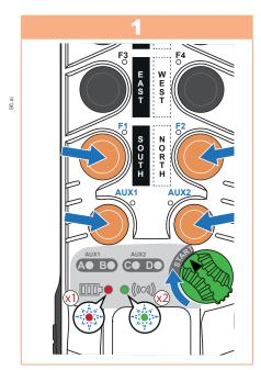
Turn **ON/OFF** switch to the **I** (ON) position. Ensure the LEDs A through D turn on and then off. Then press and hold at the same time **AUX1**, **AUX2**, **F1** and **F2** buttons and turn the **ON/OFF** switch to **START**:
