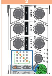
Release the **ON/OFF** switch to start pairing: LEDs A, B, C, and D light up one
