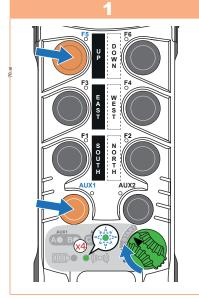
Turn **ON/OFF** switch to the **I** (ON) position. Ensure the LEDs A through D turn on and then off. Then press and hold the **AUX1 and F5** buttons and turn the **ON/OFF** switch to **START**:
