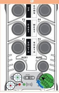
Confirm the value by turning the **ON/OFF** switch to **START**. During transmission: • Battery and radio LEDs
