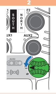
Release the ON/OFF switch and all other buttons: LEDs A and B indicate the active release mode (auto or voluntary).
