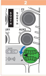
Release the **ON/OFF** switch and all other buttons to start the configuration.
