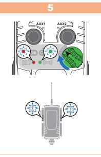
Validate the reset by tourning the **ON/OFF** switch to **START**: battery and radio LEDs flash alternatively and the receiver memorize the factory defaults (white lamp is on).
