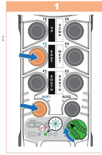
Turn ON/OFF switch to the I (ON) position. Ensure the LEDs A through D turn on and then off. Then press and hold the AUX1 and F3 buttons and turn the ON/OFF switch to **START**: • The battery LED turns off
