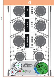
Confirm the value by turning the **ON/OFF** switch to **START**. During transmission: • Battery and radio LEDs flash alternately • Receiver light turns on.
