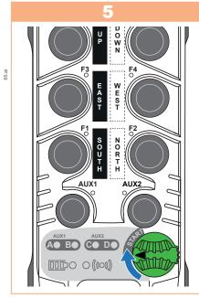
At the end of the sequence, confirm by turning the **ON/OFF** switch to **START**. **Note**: If the sequence entered is
