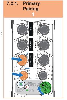
Press and hold the **AUX1 and F1** buttons and turn the **ON/OFF** switch to **START**:
