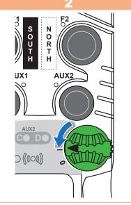
Release the **ON/OFF** switch and all other buttons to start the configuration.
