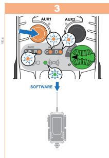
To display receiver software version press the **AUX1** button: the green radio LED turns on and the B, C and C LEDs indicate the version number (in order hundreds, tens and units).
