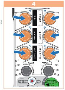
To pre-select a reset press successively the **F1**, **F2**, **F3**, **F4**, **F5** and **F6** buttons: the battery LED is blinking and all others LEDs are off.
