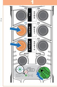
Turn **ON/OFF** switch to the I (ON) position. Ensure the LEDs A through D turn on and then off. Then press and hold the **F1** and **F3** buttons and turn the **ON/OFF** switch to **START**:
