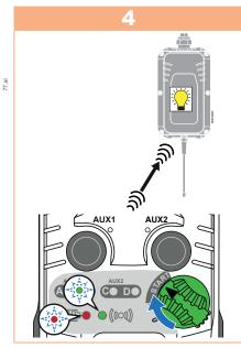
Confirm the value by turning the **ON/OFF** to **START**. During transmission: • Battery and radio LEDs flash alternately • Receiver light turns on.
