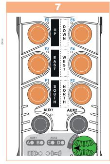
Re-enter the sequence: LEDs A and B go out after each pressing of the **F1 to F6** function buttons. Do not press any buton to clear the previous code and disable it at power up.
