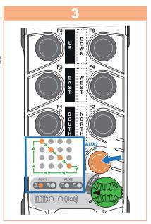
Press the **AUX2** button to start the procedure. During the scan, LEDs A, B, C, and D flash one after the other. If this LEDs sequence stops and goes to next step (4), this is due to loss communication with the receiver.
