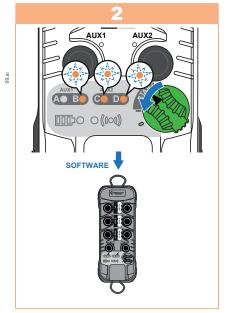
Release the **ON/OFF** switch and all other buttons, the transmitter software version is displayed (green radio LED is off):
