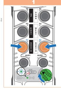
Turn **ON/OFF** switch to the **I** (ON) position. Ensure the LEDs A through D turn on and then off. Then press and hold the **F1 and F2** buttons and turn the **ON/OFF** switch to **START**:
