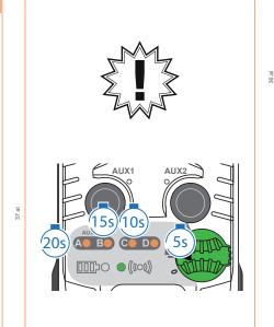
LEDs A, B, C, and D indicate the remaining time by turning off successively every 5 sec in reverse alphabetical order: D after 5 sec, C after 10 sec, B after 15 sec, and A after 20 sec.
