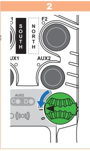
Release the **ON/OFF** switch and all other buttons: LEDs A and B indicate whether swapping is enabled or disabled.
