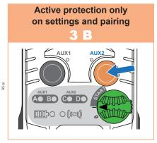
When **LED C** is off: the protection is active only on the settings and pairing functions.
