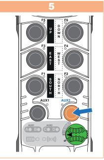
If several receivers have flashing white lights, it is possible to switch from one to the other by pressing the **AUX2** button: the preselected receiver is the one whose light flashes quickly.
