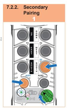
Press and hold the **AUX1 and F2** buttons and turn the **ON/OFF** switch to **START**:
