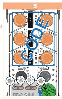
If LEDs A, B, C, and D flash at the same time, the transmitter is locked by a protection sequence. Re-enter the sequence (buttons F1-F6) and validate by turning the ON/OFF switch to START. If the code is correct, initialization starts (the green LED lights up for 2 sec).
