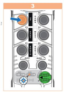
Press the **F5** button to enable the mode:
