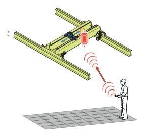
If several devices are equipped with radio controls, working in the same vicinity (e.g., in a factory), each transmitter must carry clear information that tells the operator which equipment it controls. Similarly, the operator must be able to identify the controls corresponding to the directions of movement of the equipment being steered.
