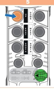
To disable the mode, press the **F5** button. This returns to the fixed radio channel setting (refer to Chapter **8.7.1**).
