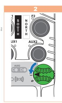
Release the **ON/OFF** switch and all other buttons to start configuration.
