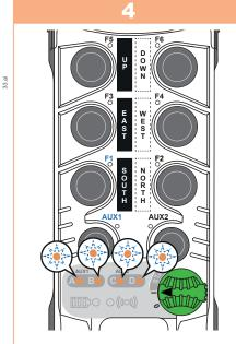
When receivers have been found, LEDs A, B, C, and D on the transmitter flash quickly.
