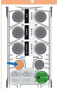
Select the desired sound level using the AUX1 button.
