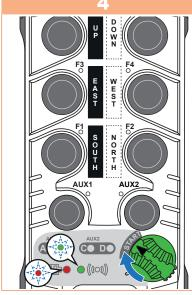
Confirm the value by turning the **ON/OFF** switch to **START**. During transmission: • Battery and radio LEDs flash alternately • Receiver light turns on.
