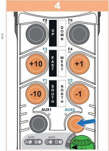
Set the desired value: • Select the unit of time using the AUX2 button (min or sec) • Re-enter the value: decrement/increment the tenths with F1/F3 and the units with F2/F5.
