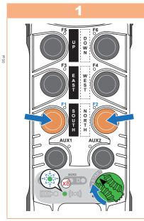
Turn **ON/OFF** switch to the I (ON) position. Ensure the LEDs A through D turn on and then off. Then press and hold the **F1 and F2** buttons and turn the **ON/OFF** switch to **START**:
