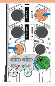
Turn **ON/OFF** switch to the **I** (ON) position. Ensure the LEDs A through D turn on and then off. Then press and hold the **AUX1** and **F4** buttons and turn the **ON/OFF** switch to **START:**
