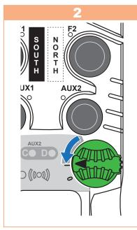
Release the **ON/OFF** button and all other buttons to start configuration. LEDs indicate the existing configuration.
