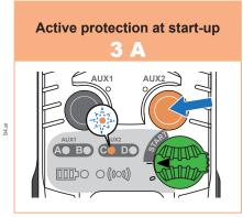
When **LED C** lights on: the protection is active au start-up.
