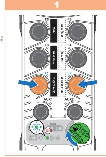
Turn **ON/OFF** switch to the I (ON) position. Ensure the LEDs A through D turn on and then off. Then press and hold the **F1 and F2** buttons and turn the **ON/OFF** switch to **START**:
