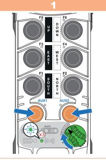
Turn ON/OFF switch to the I (ON) position. Ensure the LEDs A through D turn on and then off. Then press and hold the AUX1 and AUX2 buttons and turn the **ON/OFF** switch to **START**: • The battery LED turns off
