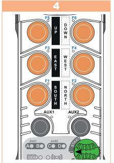
Enter the code by pressing successively on the buttons (chosen sequence): LED A turns off then on after each pressing of the F1 to F6 button. Do not press any button to clear the previous code and disable it at power up.
