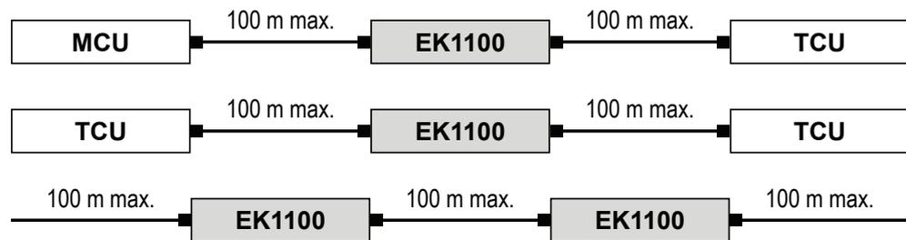
Fig. 11: Extending EtherCAT connections using EK1100 bus couplers
