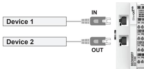
Fig. 15: Connecting EtherCAT devices (BN)
