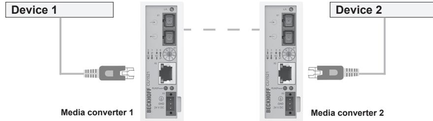
Fig. 22: Connecting EtherCAT devices (BN)
