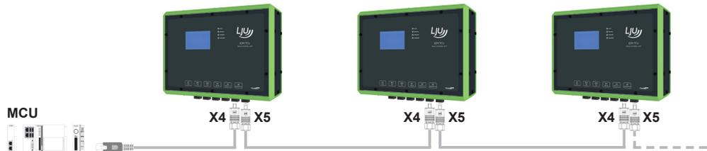
Fig. 9: Connecting the MCU and the TCUs
