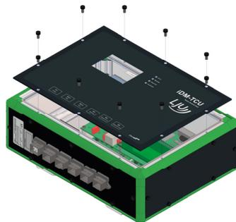
4. ➤ Disconnect the plug-in connection between the main board and the touchscreen, and remove the front panel.
