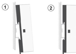
Fig. 19: Installing the CU1521 media converters <sup>(BN)</sup>
