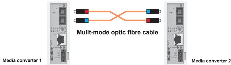
Fig. 21: Connecting the fibre optic cable <sup>(BN)</sup>
