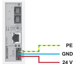
Fig. 20: Power supply of the CU1521 media converter <sup>(BN)</sup>
