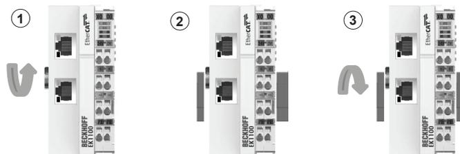
Fig. 13: Installing the EK1100 bus coupler <sup>(BN)</sup>
