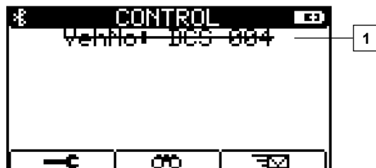
Fig. 9: BT mode set, there is no connection to a vehicle control system
