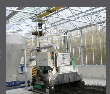
Customized solution with conductor bar, spring reel, and slip ring assembly for sludge drying systems
