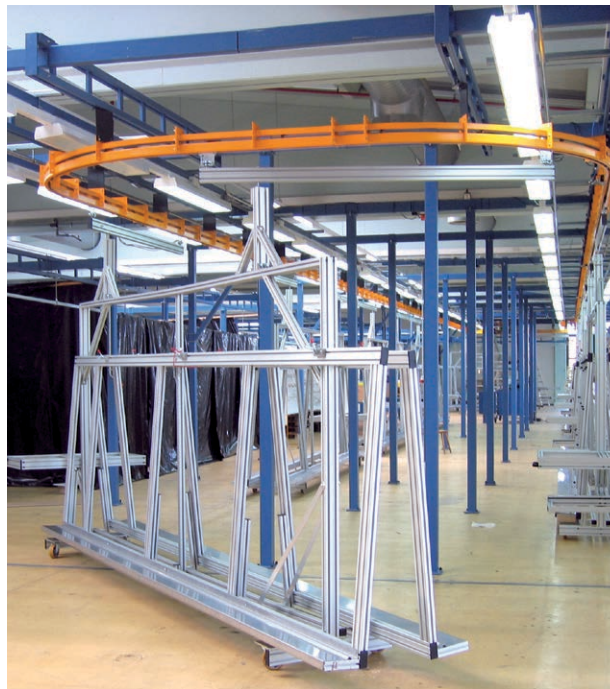
Power & Free system for the assembly of customer-specific wiring harnesses
