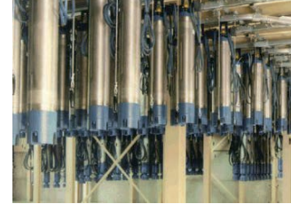
Overhead monorail system with buffer zone in a factory for submersible pumps
