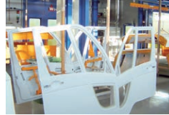
Overhead monorail system for the manual transport of vehicle components
