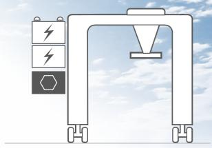
In Conductix-Wampfler Hybrid RTG systems the battery pack is the main power supply and connected through a very efficient DC/DC converter to the DC bus of RTG drive.
